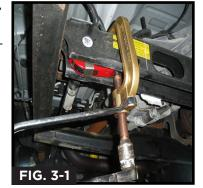
5. Reinstall torsion bar adjustment bolt, thread the bolt in until it makes contact with the MAXXCam torsion bar key.
