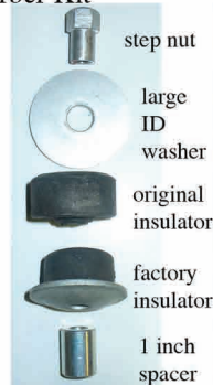
B. Assemble above parts in order shown
